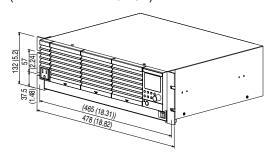
When mounting on a millimeter rack (Bracket model: KRB150-TOS)
