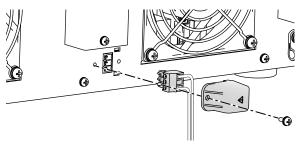
Connect the N SENSE terminal of the product to the N terminal of the load using sensing cables. Likewise, connect the L SENSE terminal to the L terminal on the load.
