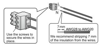
Attach the connector and SENSE terminal cover.
