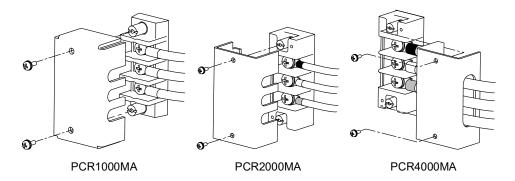
Attach a crimping terminal to the switchboard end of the power cord.
