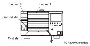
While pressing up on the bottom tab of louver B, pull it towards you. Slide the entire louver down, and remove the louver from the panel.
