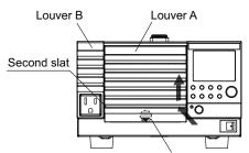
Fix the pin inside the louver in place.
