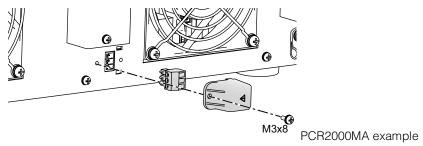
**3** Connect the sensing cables to the connector.
