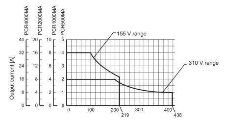
If you use the product with a current that exceeds the rated DC output current, the protection functions will be activated, which may cause the output voltage to drop or turn off the output.
