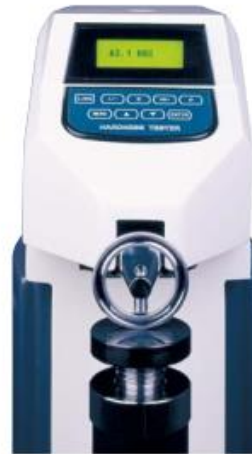
Protrudent design for testing in place difficult to reach
