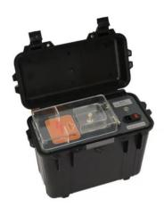
It is working together with GD-4133 Cable Fault Detector, used for detecting high impedance leak fault, flashover fault, low impedance earth and open circuit fault of power cables. GD-4133S supplied pulse coupling signal for GD-4133 and isolate it from high voltage equipment.
