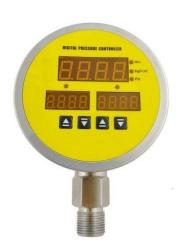
This three-screen digital display electric contact pressure gauge is mainly to replace the traditional mechanical electric contact pressure gauge, so the output control method is the same as the traditional mechanical electric contact (a common line, a high alarm, a low alarm). The user can connect the wires according to the wiring method of the mechanical electrical contact pressure gauge.
