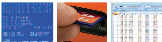
Backlit LCD displays numerical values. The data can be stored in SD memory card (included) and then transferred from meter to PC using Excel ® software and datalogged readings.
