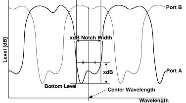
Obtain the width (xdB\_Notch\_Width) between the two points, which are above the bottom level of each channel by the parameter THRESH\_LEVEL, and its center wavelength (Center\_Wavelength).
