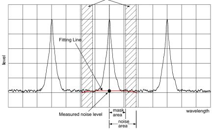
Data range for use in the fitting calculation
