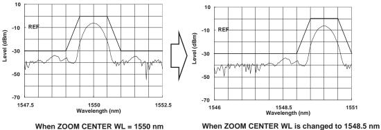
(template also moves in synch with the waveform)
