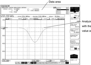
Analyzes the waveform with the maximum level value as a referemce.
