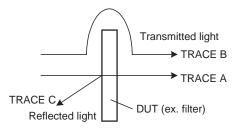
The value of k is an absorption coefficient which is used in determining the DUT reflectivity and transmission efficiency. Different algorithms are used depending on whether transmission efficiency or reflectivity is estimated, so the k value also varies accordingly.
