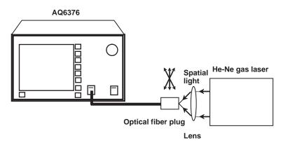
The sweep width is set to 0 nm, the center wavelength is fixed, and measurement of the single-wavelength light only is taken. Finely adjust the optical fiber plug while observing the displayed waveform so as to set the light source input level to the peak.
