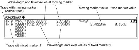
Moving marker Ø. SENS: HIGH1/CHOP 11 11 RES: nm AVG: н 2 6000nm 5000nm OdBm UdBM )000nm юыв Number displayed on fixed marker
