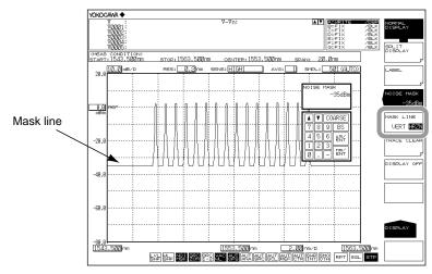
Displays the waveform with level values at or below the mask value as the mask value.
