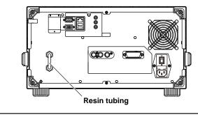
The recommended purge gas flow rate into the AQ6376 is 15 to 20 SCFH (7 to 9.5 L/ min).
