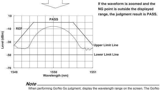
Go testing process is not performed on wavelength ranges that are not displayed.
