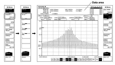
Example of a measured waveform of an FP-LD
