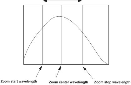
Wavelength display sweep span
