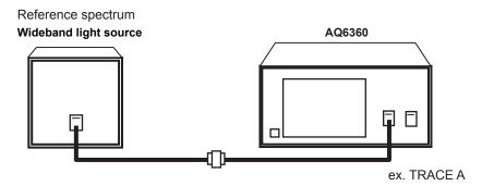
Spectrum measurement after passing through the filter
