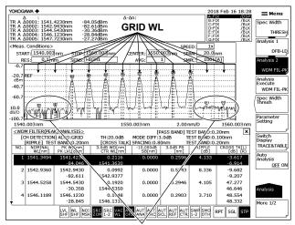
Grid wavelengths are detected as channels.
