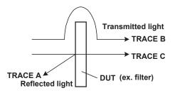
(2)Estimating the reflectivity (trace C) from the transmitted light spectrum (trace A) Reflected light spectrum (TRACE C) = 1-k (TRACE A/TRACE B)
