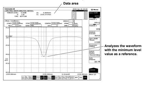
Notch width measurement waveform (BOTTOM)
