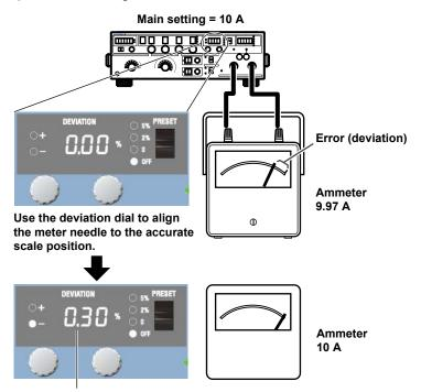
Setup example: Main setting = 10 A, divider value n/m = 1
