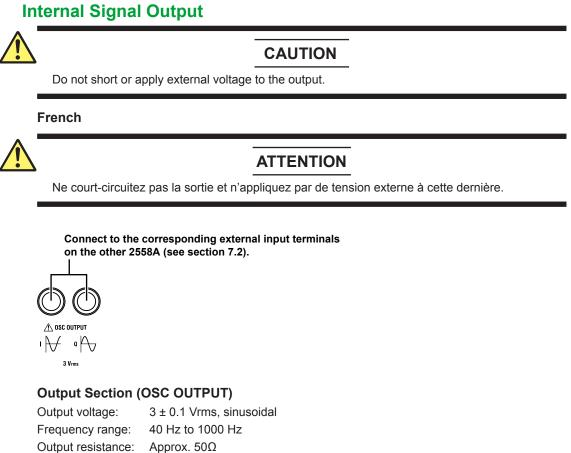
If the frequency is set to EXT1 or EXT2, these terminals output the signal connected to EXT OSC INPUT.
