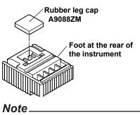
If you attach the front rubber leg cap, you will not be able to stack the 2558A.
