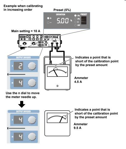
In the above example, the 2558A is generating –5.00% of the output setting. To calibrate the scale, turn a deviation dial to move the meter needle to the correct position. For details on how to read the deviation, see "Deviation" on the previous page.
