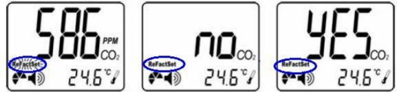
Using this function deletes all stored settings and sets the device back to factory default settings. This might be reasonable if the calibration has not been done properly, for example.
