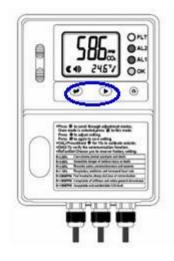
The gas detector has an automatic lock function to prevent the settings from being changed unintentionally. If you wish to adjust the settings you have to unlock the device first. To do so, press and hold the "Mode" key and the "Enter" key at the same time for 5 seconds. Now the device is unlocked and you can change the settings. After 30 minutes, the device will be locked again. To activate the lock function manually, press and hold the "Mode" and "Enter" key once again for 5 seconds.
