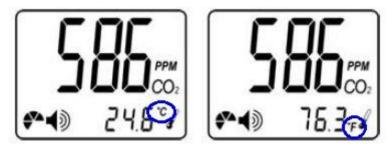
To switch between "°C" and "°F", press the "Enter" key.
