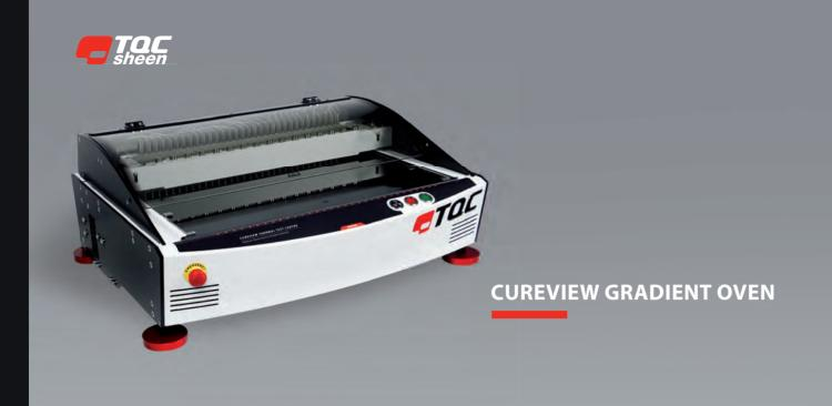
The CureView Gradient Oven is a flexible oven that allows the user to heat up test panels on a glass bed to a variety of temperature profiles, varying from ambient +5°C to 350°C/ ambient +41°F to 662°F. Elevated temperatures are instantly generated by 32 spectral filtered IR halogen heaters, which can be controlled individually and allow the setting of any form of
