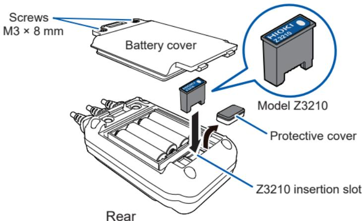
To maintain the dust-proofness and water-proofness, put the protective cover on the Z3210 insertion slot regardless of the presence or absence of the Z3210.
