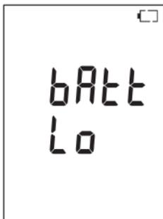
When the indicator shows no remaining battery power (the
