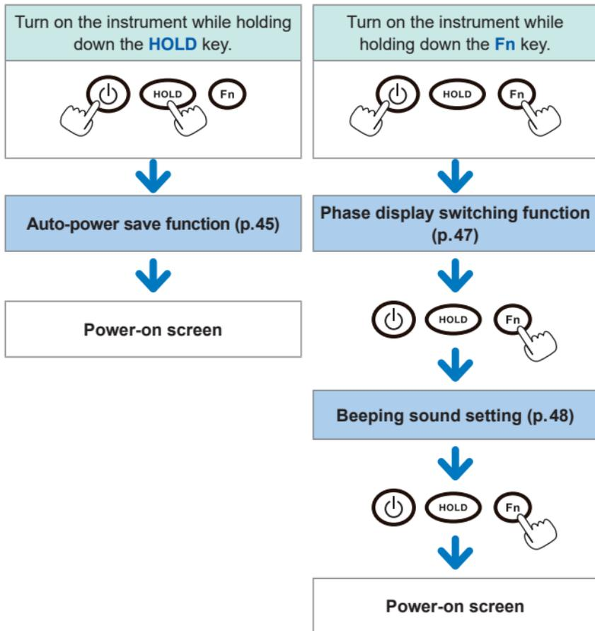
Turn on the instrument while holding down the **HOLD** and **Fn** keys.
