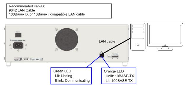
If the lamp does not turn green when you connect a LAN cable, the instrument or connected device may be malfunctioning, or there may be a wire break in the LAN cable.
