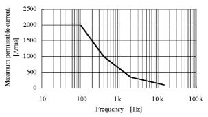
Fig.3 Frequency-dependent deletion characteristics
