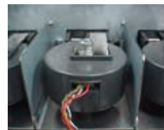
DCCT current sensor (in the PW3337)
